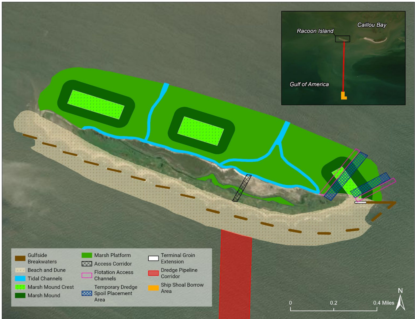
Figure 2-9. Raccoon Island Restoration Project Alternative 2 Features (including two potential northeastern flotation access channel options [Option 1 – eastern; Option 2 – western]).
