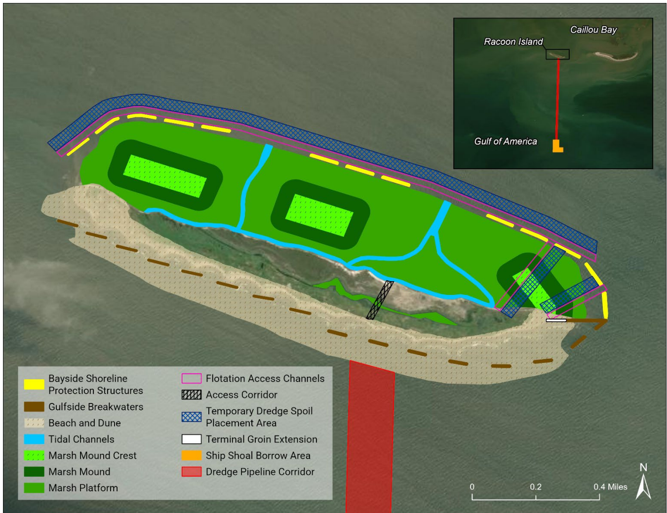
Figure 2-10. Raccoon Island Restoration Project Alternative 3 Features (including two potential northeastern flotation access channel options [Option 1 – eastern; Option 2 – western]).
