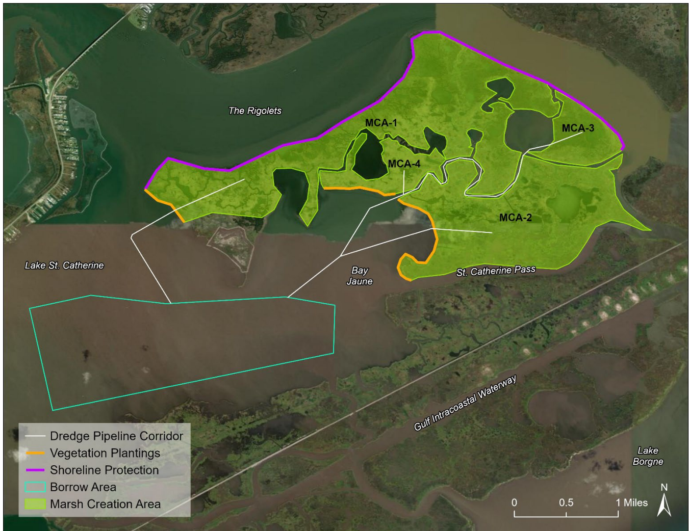
Figure 2-3. East Orleans Landbridge Restoration Project Alternative 2 Features.
