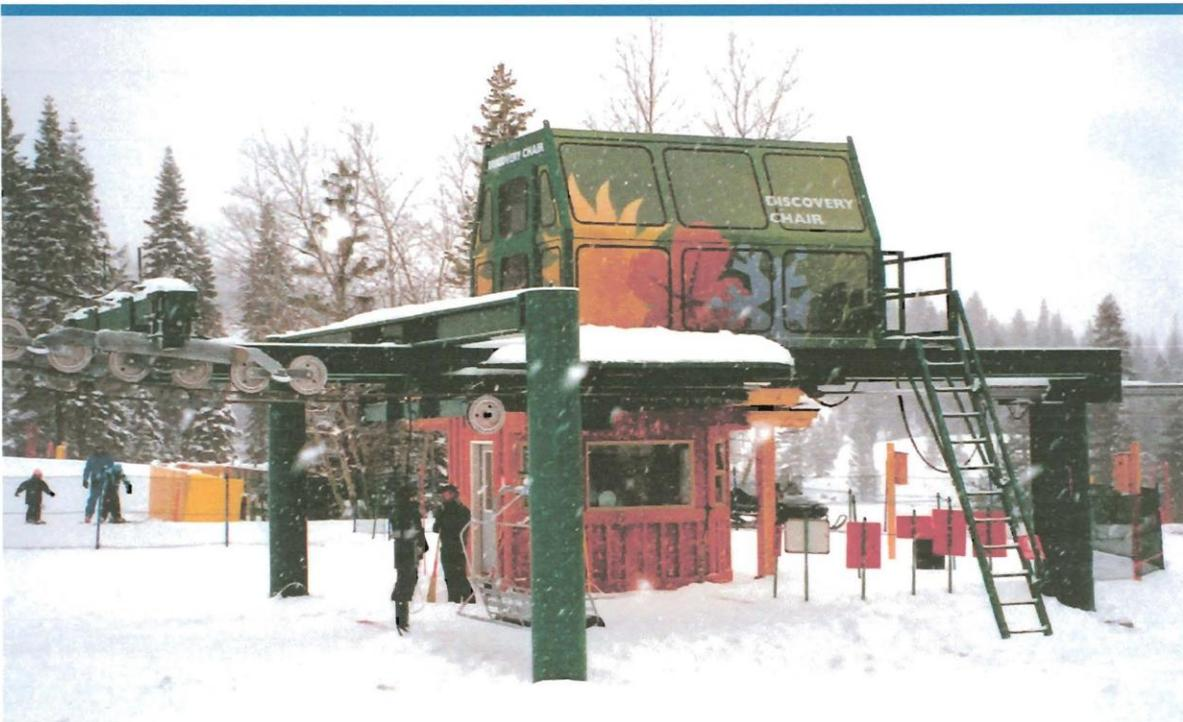
The SPRINT light-duty drive and tension drive terminals, when combined with either the Eclipse or Pegasus return terminals, creates a smooth running, economical system that fits the needs of beginner and intermediate terrain requirements. The Doppelmayr CTEC SPRINT fixed grip drive terminals are known especially for their time-proven technology, long service life, ultra low maintenance and high capacities.
