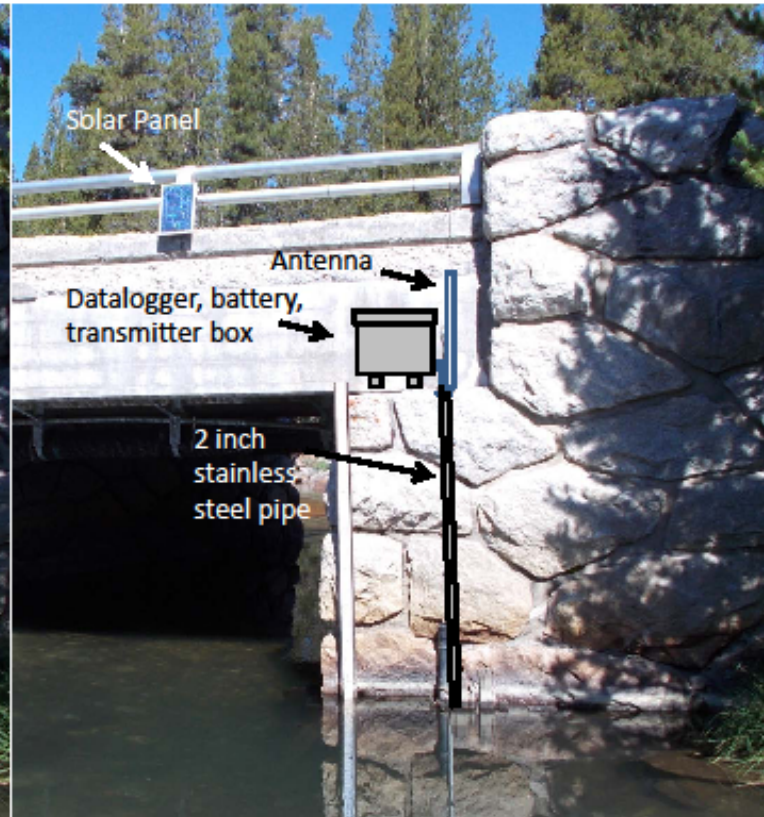
Proposed Gage Installation Mockup (staff plate and solar panel would remain; the battery box could be mounted under the bridge)
