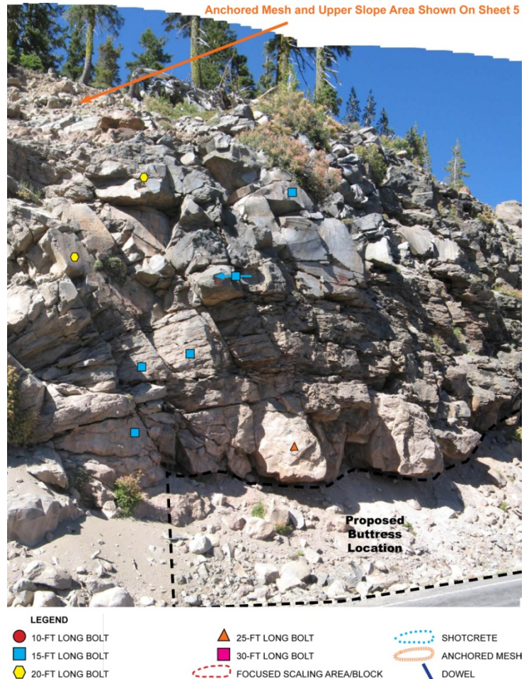
FIGURE 8. ANDERSON POINT ROCKFALL MITIGATION TREATMENTS
