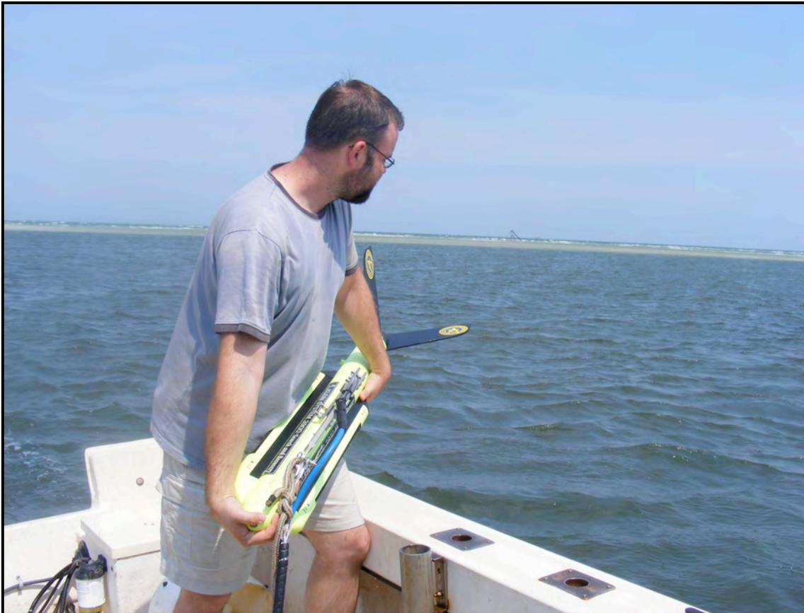
**Figure 6. Deploying the KLEIN 3900 digital sidescan sonar.**
