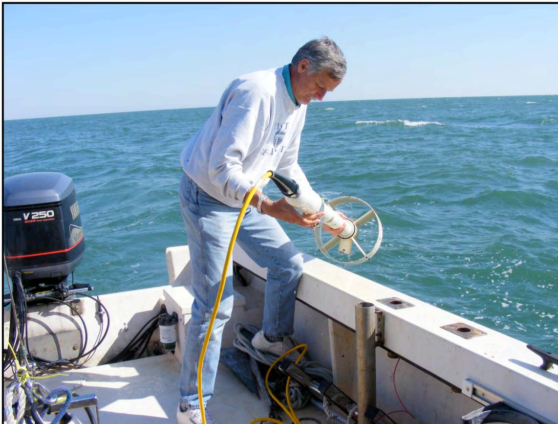
**Figure 5. Deploying EG&G GEOMETRICS G-881 cesium vapor magnetometer.**
