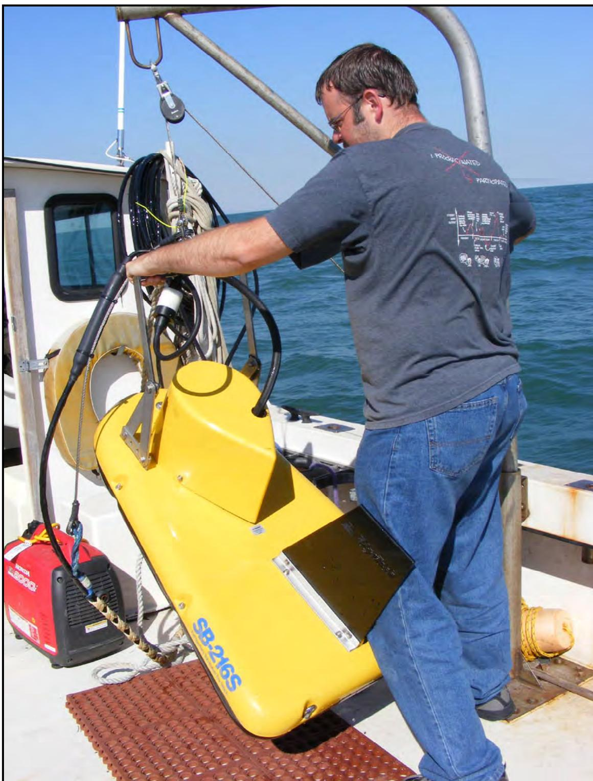
**Figure 7. Deploying the EDGETECH sub-bottom 216S tow vehicle.**
