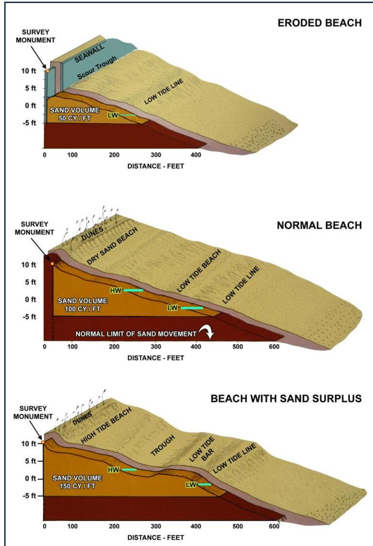
**FIGURE 2.8.** The concept of unit-width profile volumes for a series of beach profiles showing an eroded beach with a deficit, a normal beach, and a beach with a volume surplus. Profile volumes integrate small-scale perturbations in profile shape and provide a simple objective measure of beach condition. Indicated quantities are realistic for many East Coast beaches within the elevation limits shown. [After Kana 1990]
