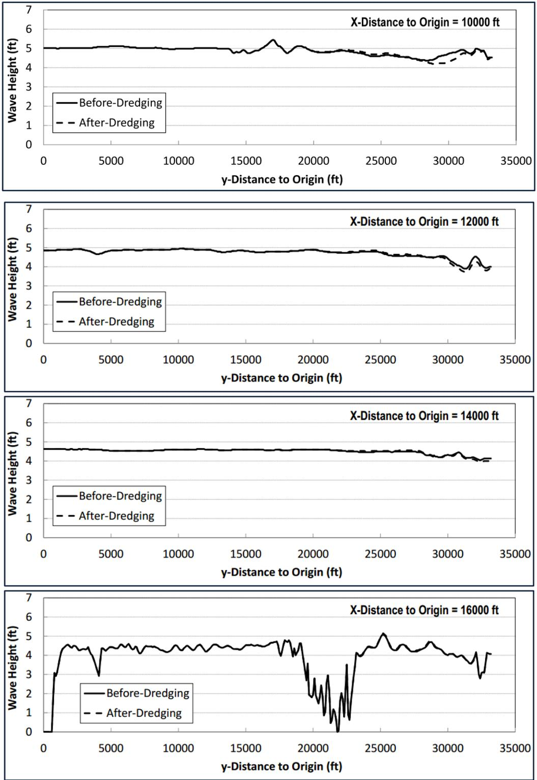
**FIGURE 3.17(5-8).** STWAVE simulated wave height comparisons at different vertical cross-sections parallel to the “y” axis (ie – with constant distance to the origin in the “x” direction) as illustrated in Figure 3.14.
