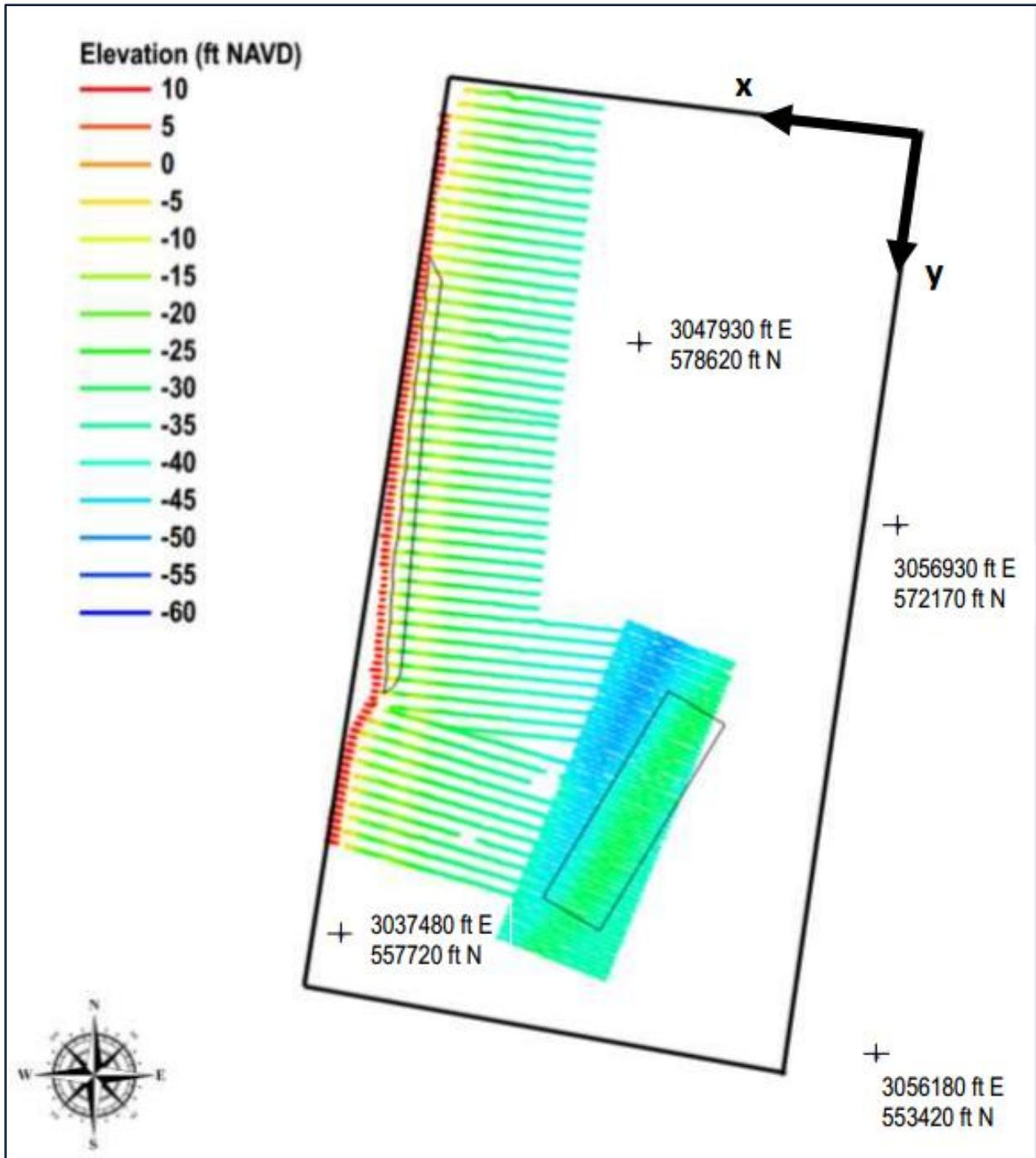
**FIGURE 3.6.** Bathymetric data collected by CSE in October 2014. To illustrate the relative coverage of bathymetric data to wave model computational domain, the thicker black lines in the figure represent the wave model computational domain and the thinner black lines represent the proposed beach fill and designated borrow area.
