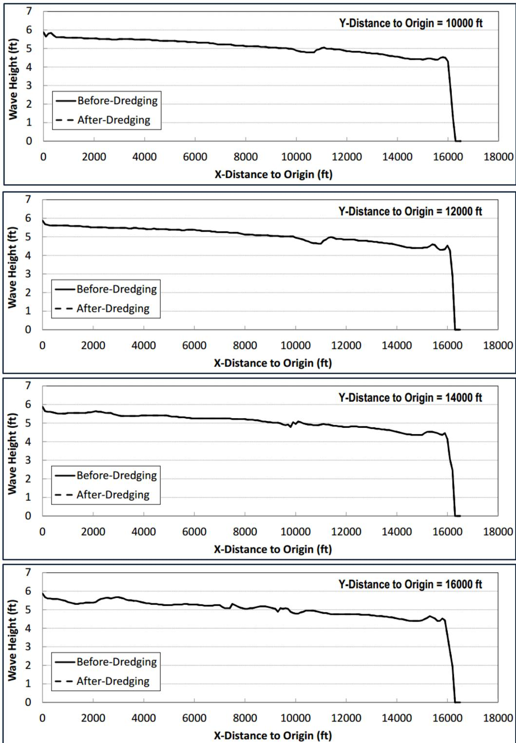
**FIGURE 3.16(5-8).** STWAVE simulated wave height comparisons at different horizontal cross-sections parallel to the “x” axis (ie – with constant distance to the origin in the “y” direction) as illustrated in Figure 3.14. “0” is the offshore model boundary and the shoreline is at the right side of the graph.
