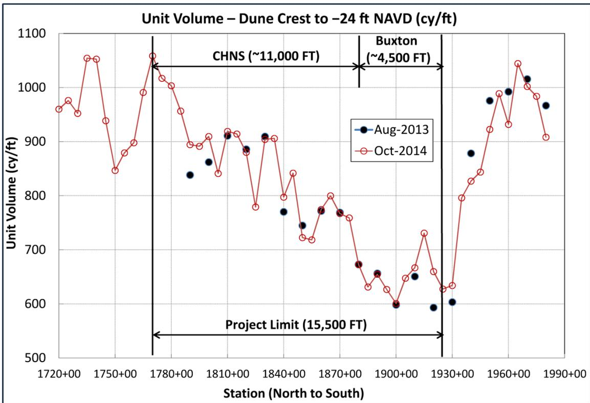
**FIGURE 2.13.** Variation in unit volume along the Buxton project shoreline between the foredune and -24 ft NAVD. October 2014 data were collected every 500 ft alongshore with profiles offset ~60 ft from the August 2013 data.
