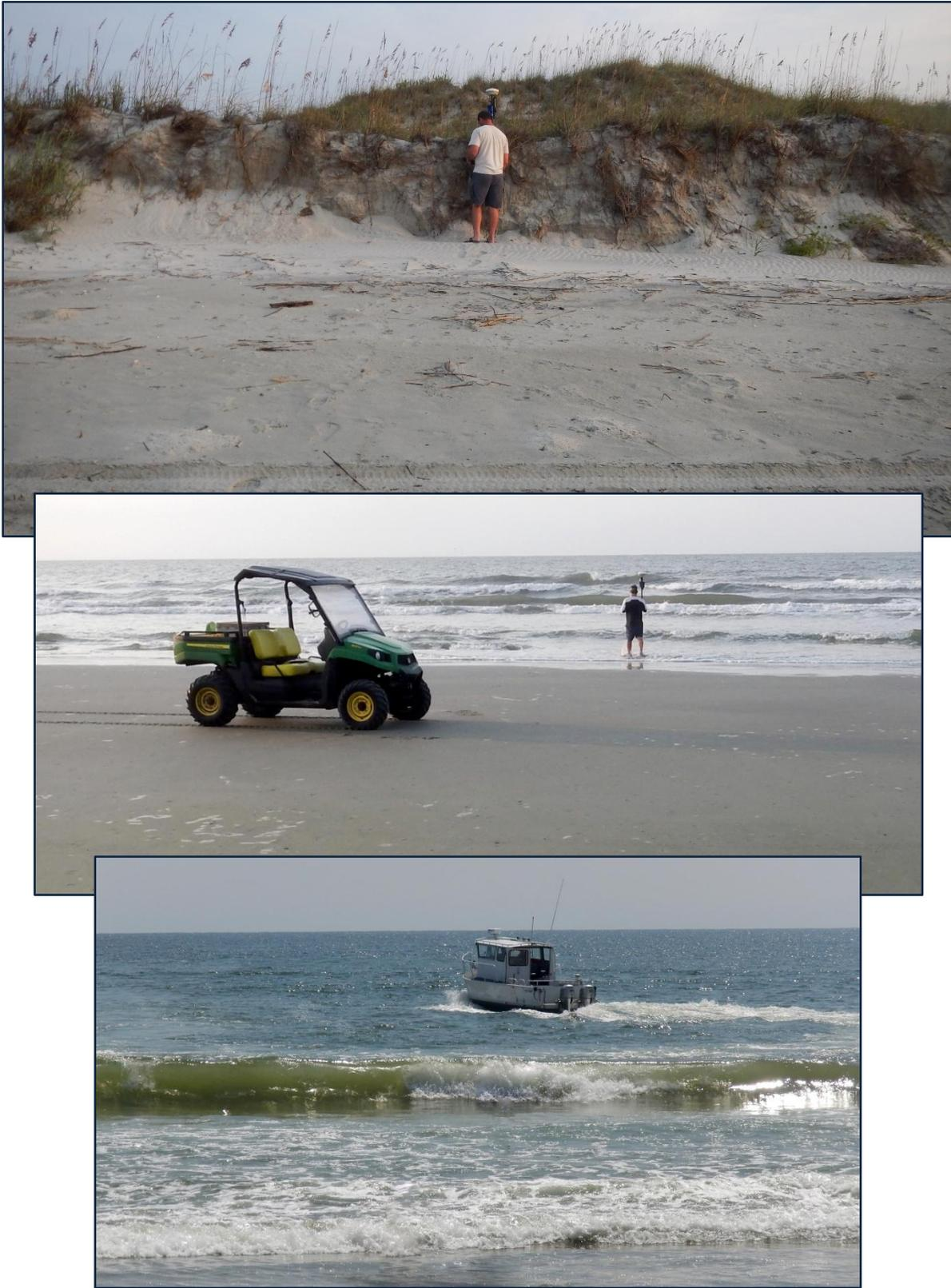
**FIGURE 2.3.** Field data collection methods involved subaerial survey using RTK-GPS at low tide and hydrographic surveys by boat at high tide. Fieldwork for Buxton was completed in August 2013 and October 2014.
