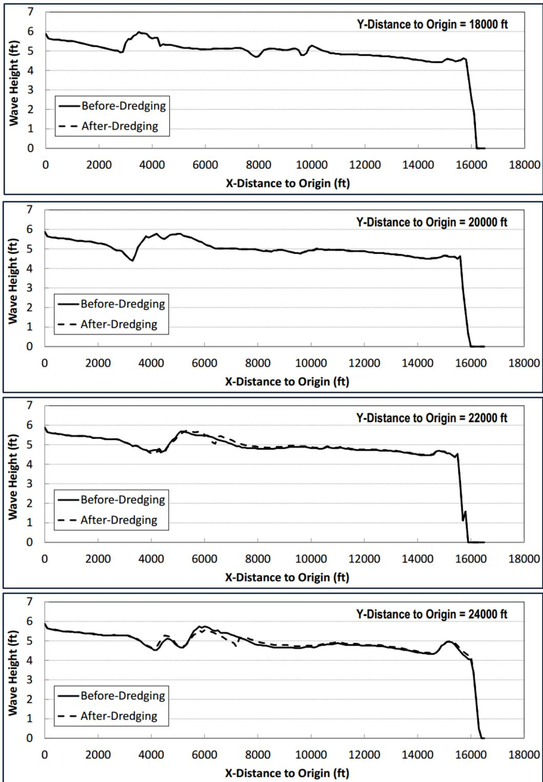
**FIGURE 3.16(9-12).** STWAVE simulated wave height comparisons at different horizontal cross-sections parallel to the “x” axis (ie – with constant distance to the origin in the “y” direction) as illustrated in Figure 3.14. “0” is the offshore model boundary and the shoreline is at the right side of the graph.
