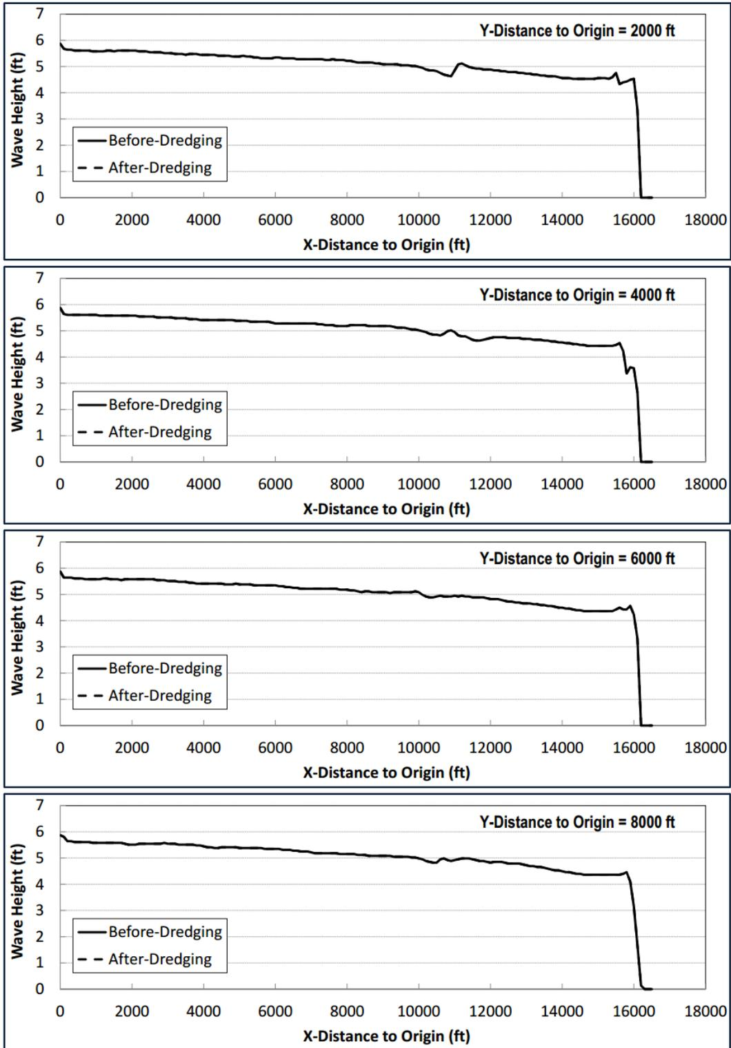
**FIGURE 3.16(1-4).** STWAVE simulated wave height comparisons at different horizontal cross-sections parallel to the “x” axis (ie – with constant distance to the origin in the “y” direction) as illustrated in Figure 3.14. “0” is the offshore model boundary and the shoreline is at the right side of the graph.
