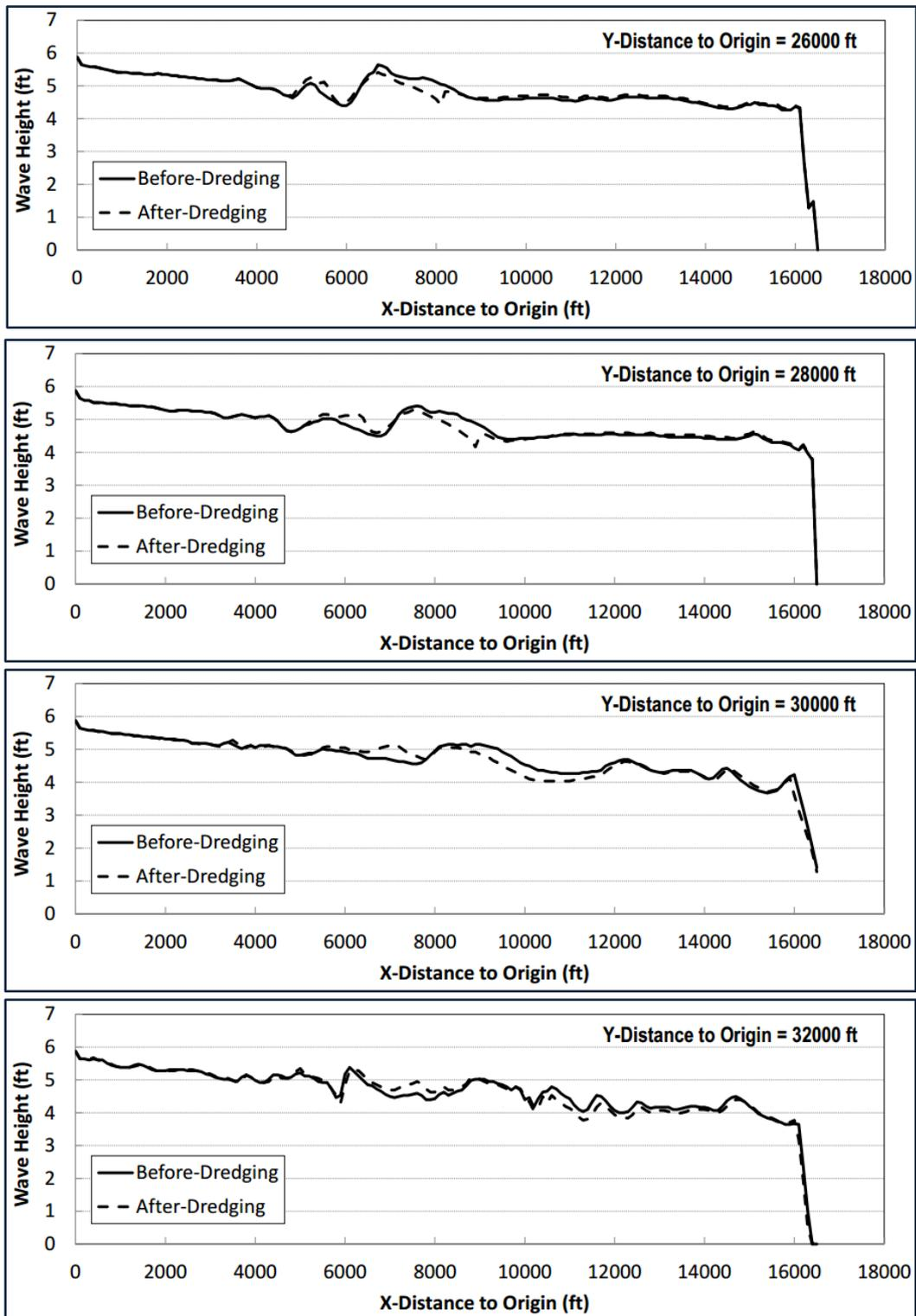
**FIGURE 3.16(13-16).** STWAVE simulated wave height comparisons at different horizontal cross-sections parallel to the “x” axis (ie – with constant distance to the origin in the “y” direction) as illustrated in Figure 3.14. “0” is the offshore model boundary and the shoreline is at the right side of the graph.
