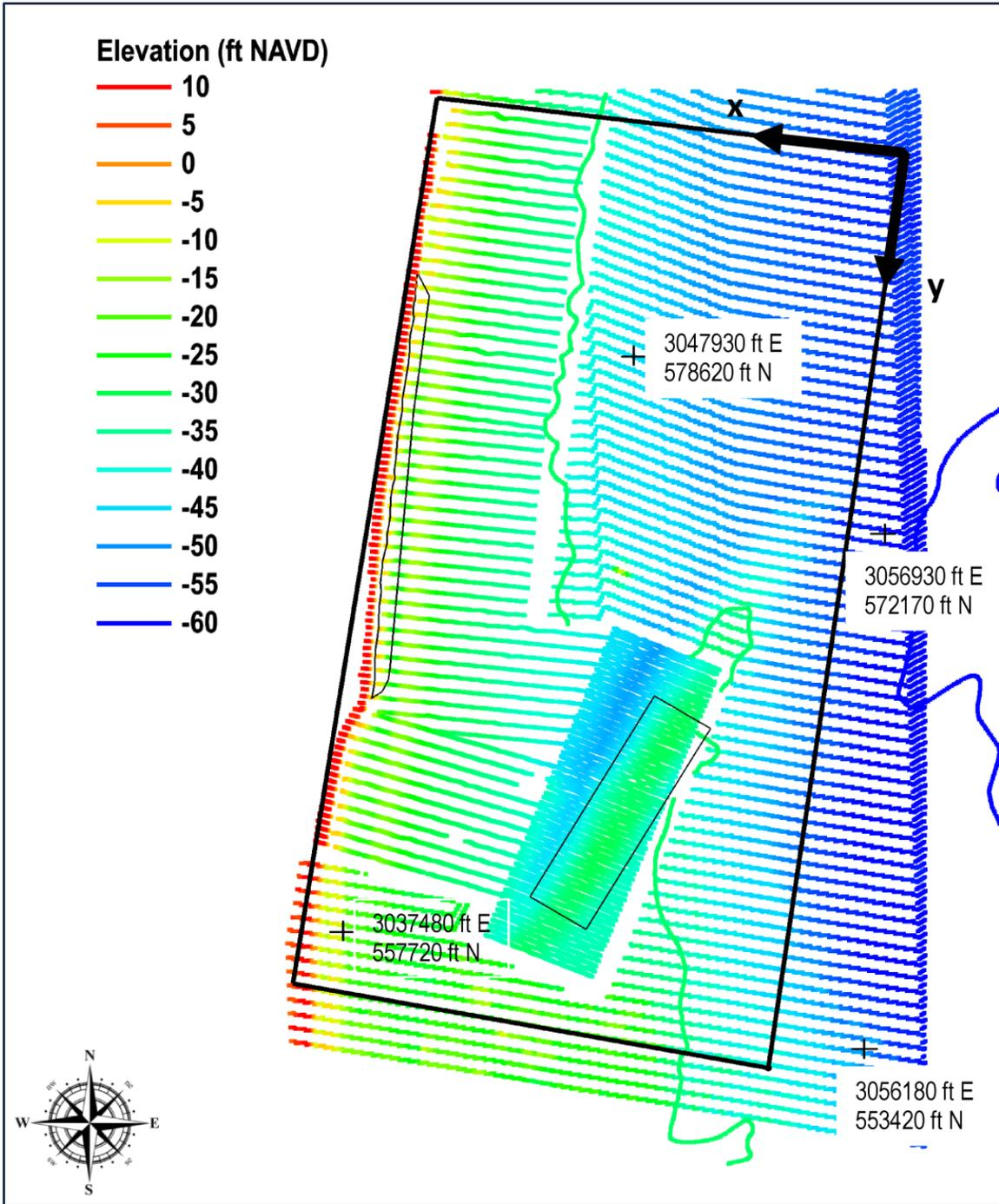
**FIGURE 3.8.** Combined bathymetric data used in the wave model for pre-project condition (ie – before dredging). To illustrate the relative coverage of bathymetric data to wave model computational domain, the thicker black lines in the graphic represent the wave model computational domain, and the thinner black lines represent the proposed beach fill and designated borrow area. The shoreline is on the left side of the graphic.
