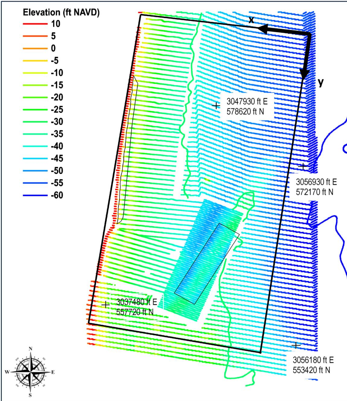
**FIGURE 3.9.** Combined bathymetric data used in the wave model for post-project condition (ie – after dredging). Excavation of 7 ft is assumed in the designated borrow area. It represents the biggest impact that dredging may cause to the project area. The shoreline is on the left side of the graphic.
