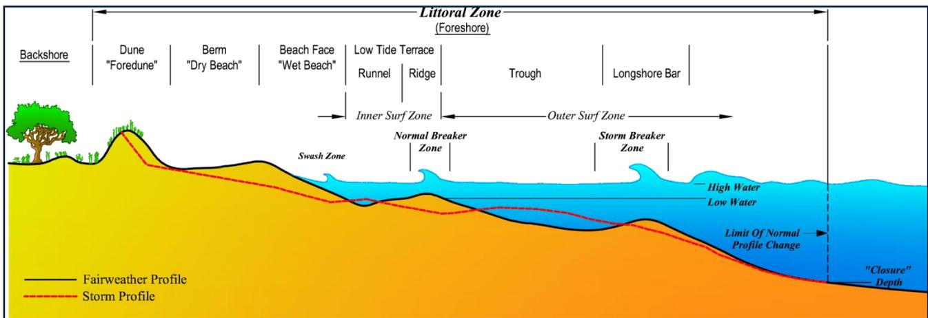
**FIGURE 2.6.** Representative profile of the littoral zone illustrating the principal features between the dune and offshore. The profile varies with changes in wave energy, the passage of storms, and differences in sediment quality. The Buxton erosion analysis takes into account the cycle of beach profile changes and focuses on the sand volumes in the entire littoral zone. [Based on Komar 1998]
