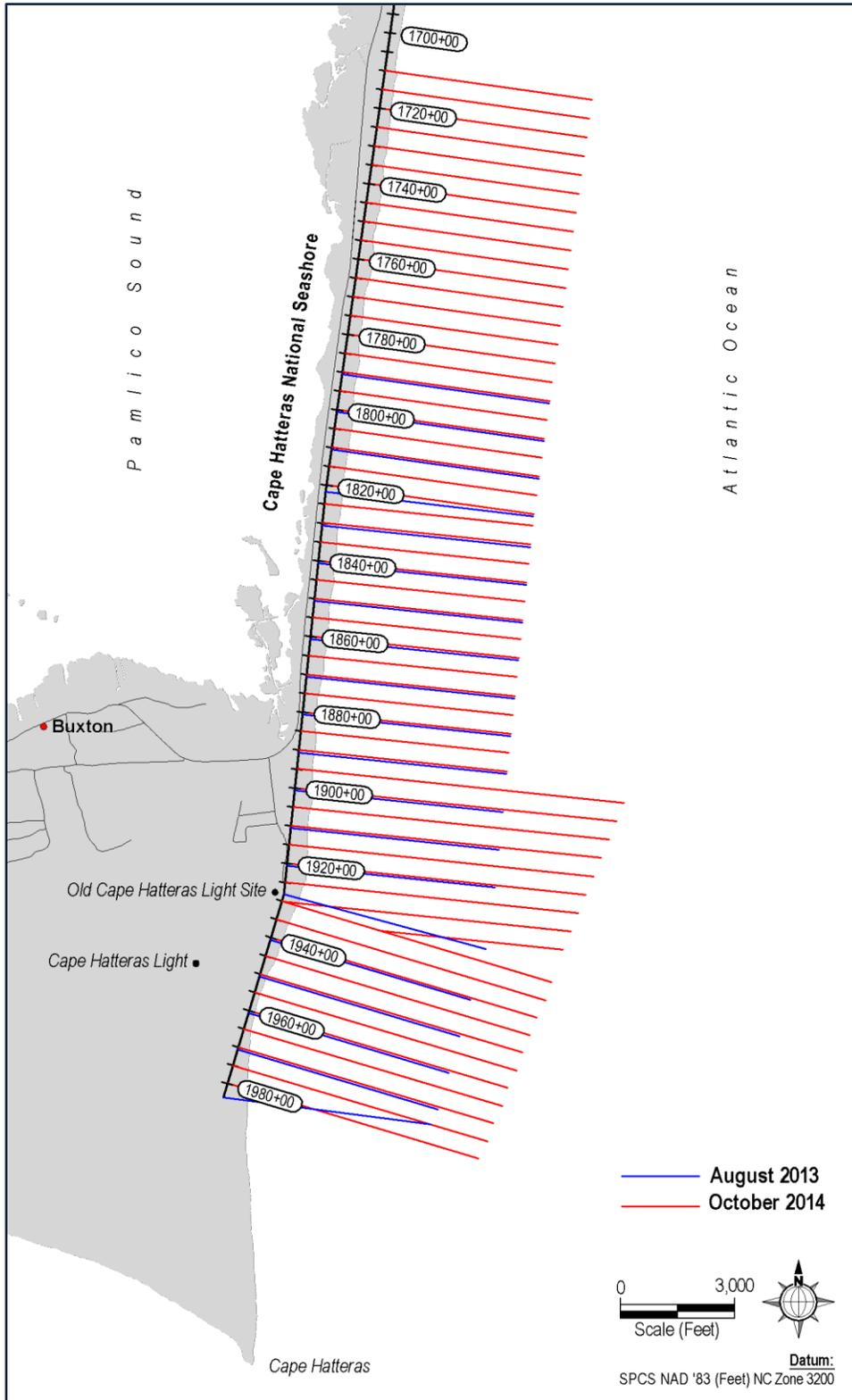
**FIGURE 2.1.** CSE’s baseline, profile stationing, and profile azimuths for the Buxton area. Phase 1 profiles (August 2013) fell on odd-numbered stations for reasons given in the text. Phase 2 profiles at 500-ft spacing (October 2014) are positioned at even-numbered stationing for future convenience.
