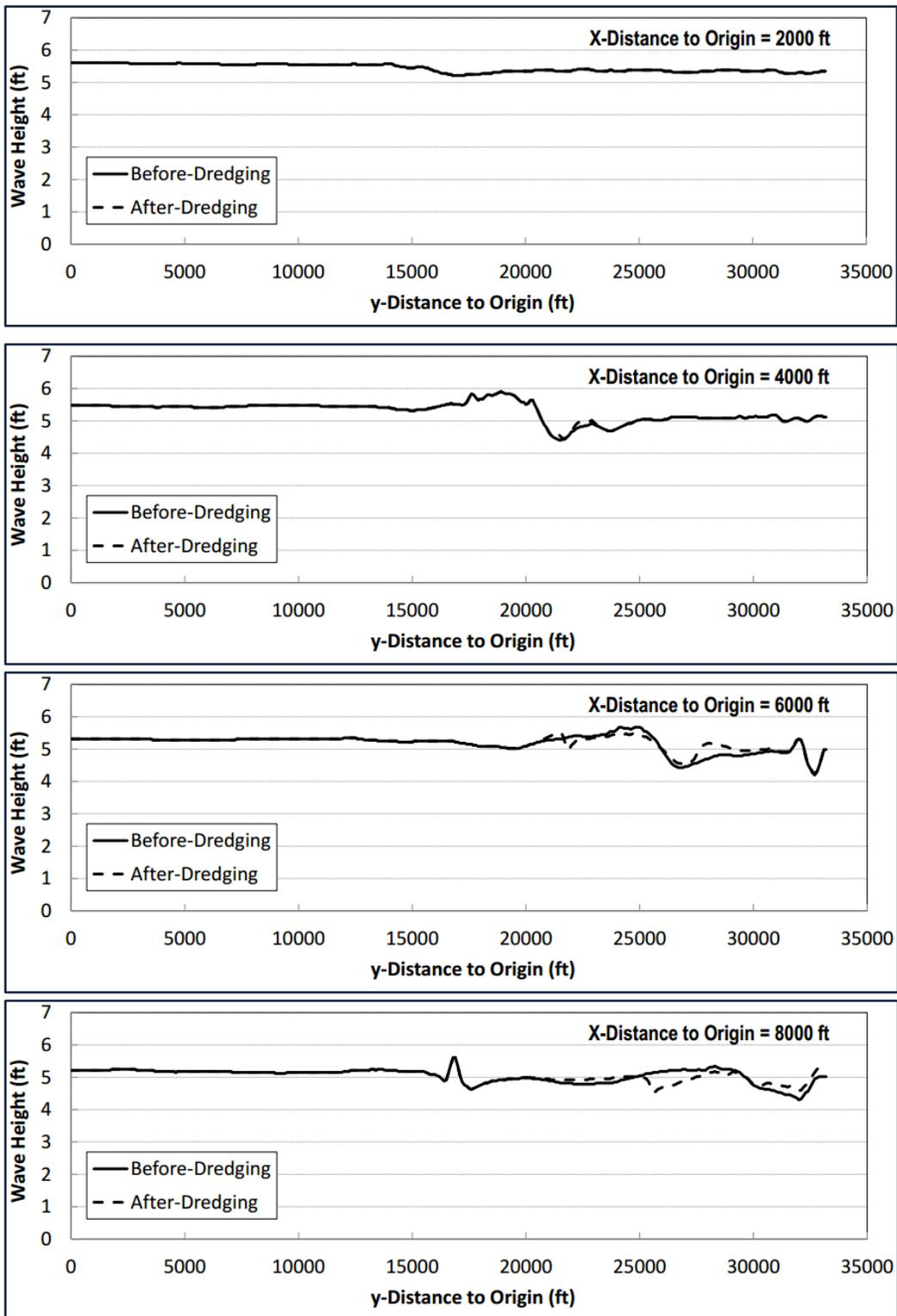
**FIGURE 3.17(1-4).** STWAVE simulated wave height comparisons at different vertical cross-sections parallel to the “y” axis (ie – with constant distance to the origin in the “x” direction) as illustrated in Figure 3.14.
