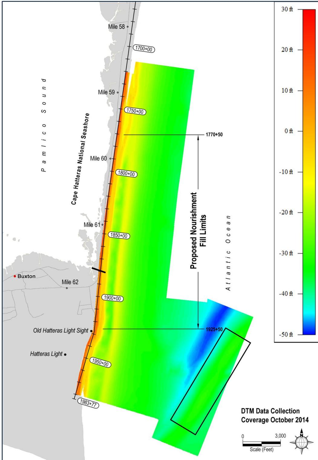
**FIGURE 2.4.** Color-coded topography and bathymetry DTM interpolated from the October 2014 survey for the Buxton project area. Note variations in water depth (and profile geometry) between the outer bar and the beach. The “salient” in the shoreline between stations 1890+00 and 1980+00 is sand retained by groins at the old Cape Hatteras Lighthouse site. The alignment of the offshore bar is straighter than the shoreline north and south of the salient.
