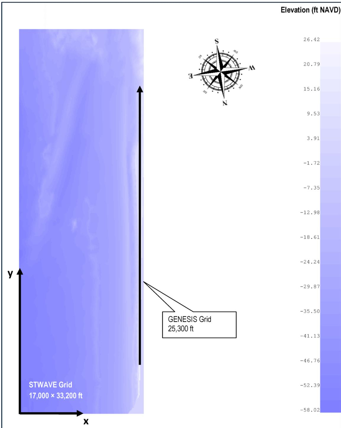
**FIGURE 3.10.** Model grid and interpolated bathymetry for before-dredging scenario. See Figure 3.8 for model origins and “x” and “y” axes. Notice the orientation of north indicated on the graphic. The shoreline is on the right near the GENESIS grid in this graphic.
