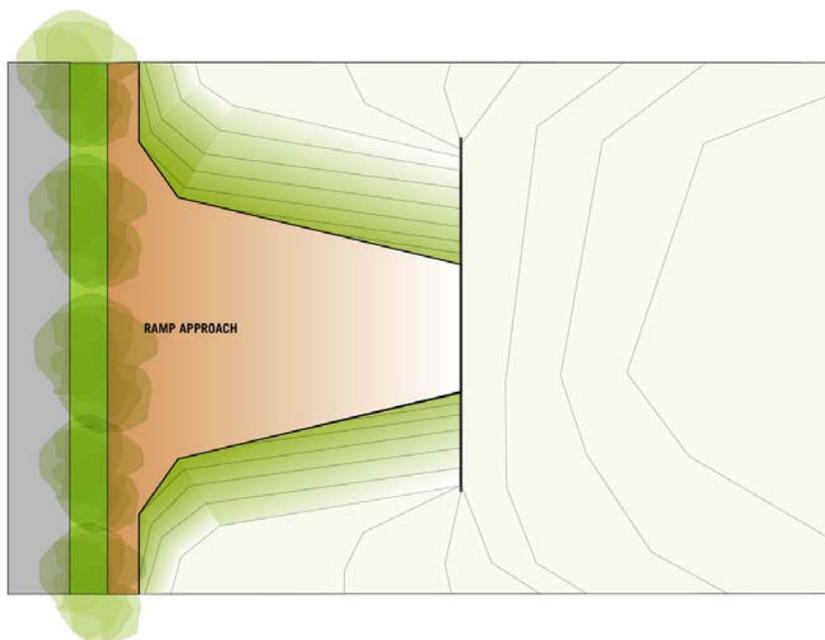
NOTE: These graphics illustrate the design strategy for the entrance to the underground Center. As shown in the top graphic, the gentle slope of the ground would be used to shield the entrance from surrounding views except for those directly in front of the facility. As shown in the bottom graphic, the entry ramp would be flanked by sloping terrain so that it would seem that a visitor is entering the side of a hill rather than descending underground.
