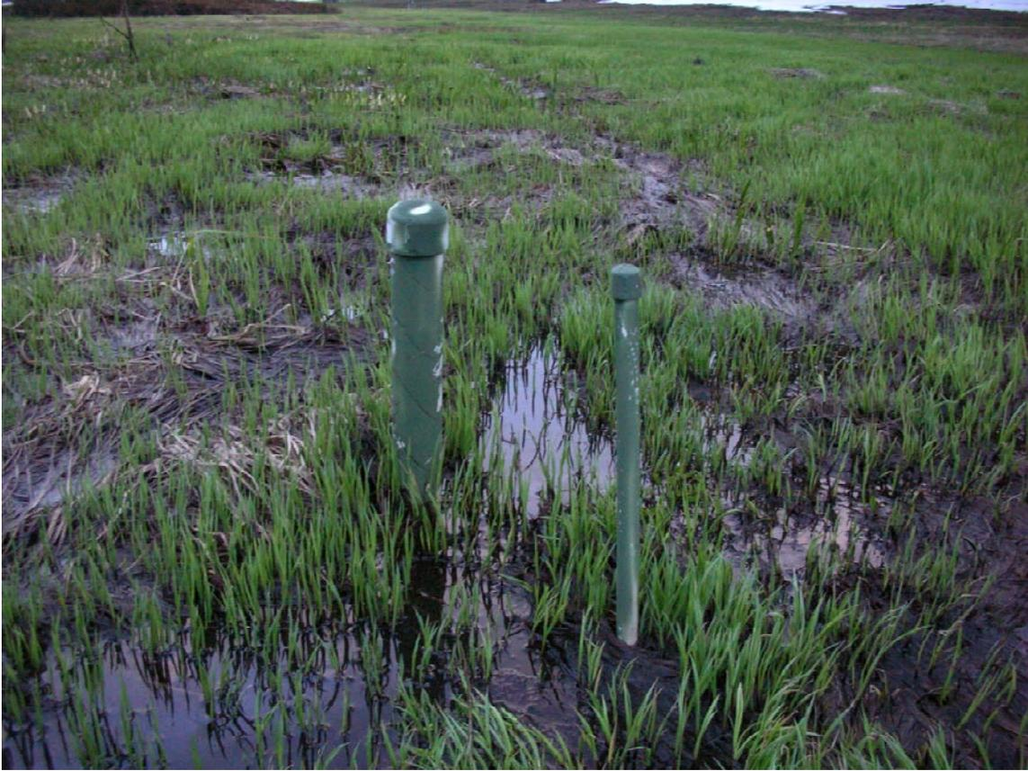
**Photo 1 Groundwater monitoring well (2-inch PVC) and piezometer (1/2-inch PVC) installed in Crane Flat meado**
