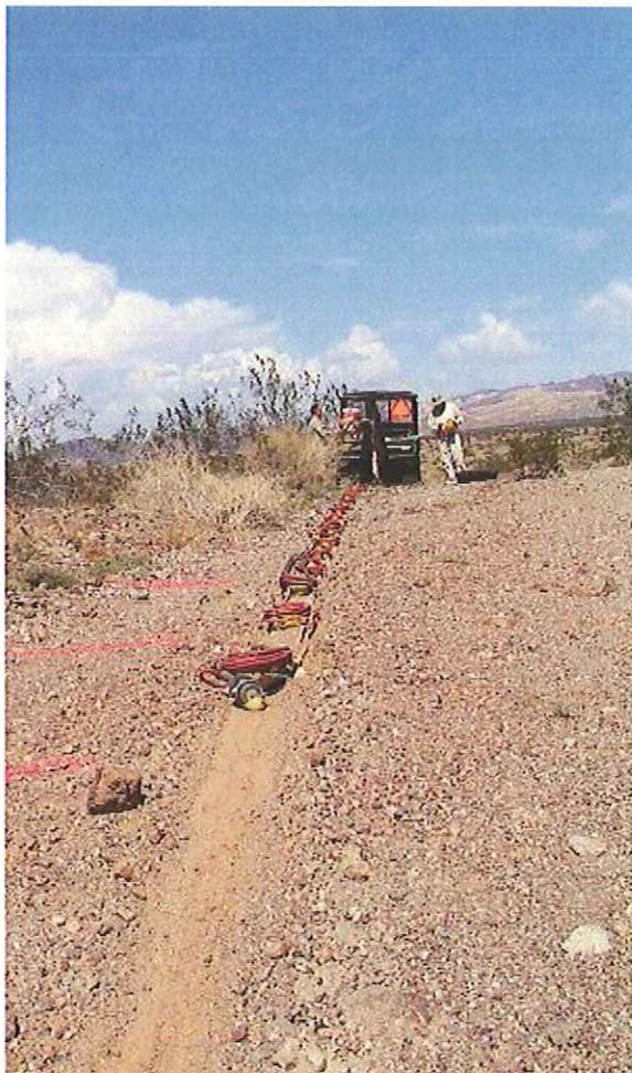
**Figure 2 - Towed Geophone Array**
