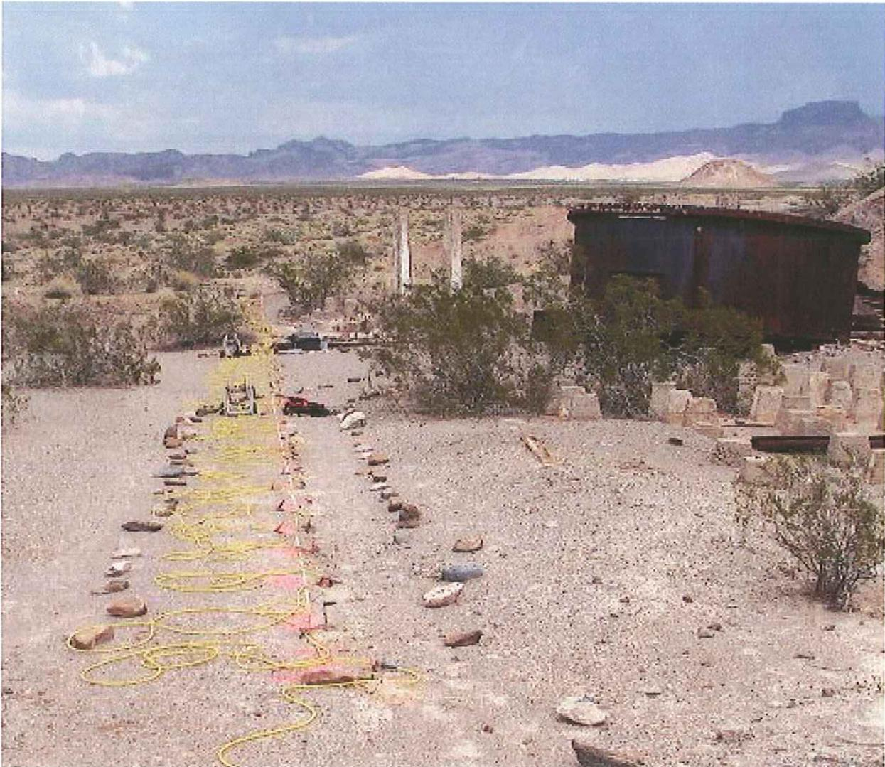
**Figure 1 - Electrode Array**
