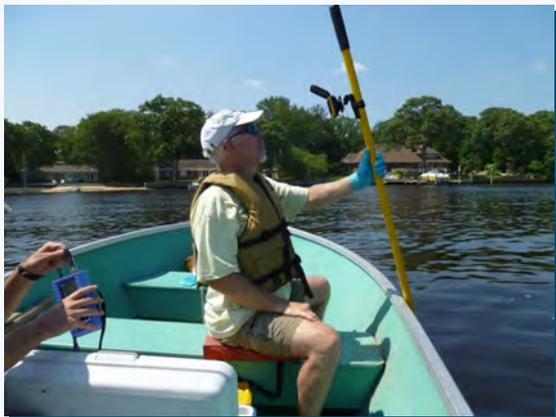
Figure O-2a. Aqua-vu underwater camera
