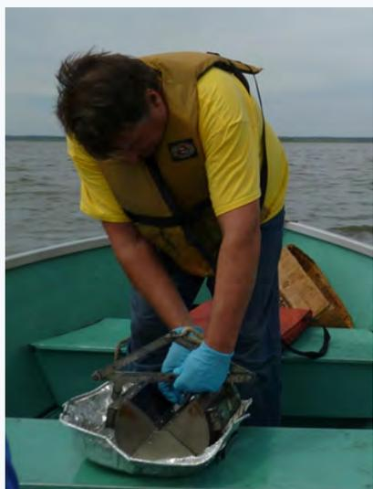
Figure O-2c. Ponar dredge sediment sampler
