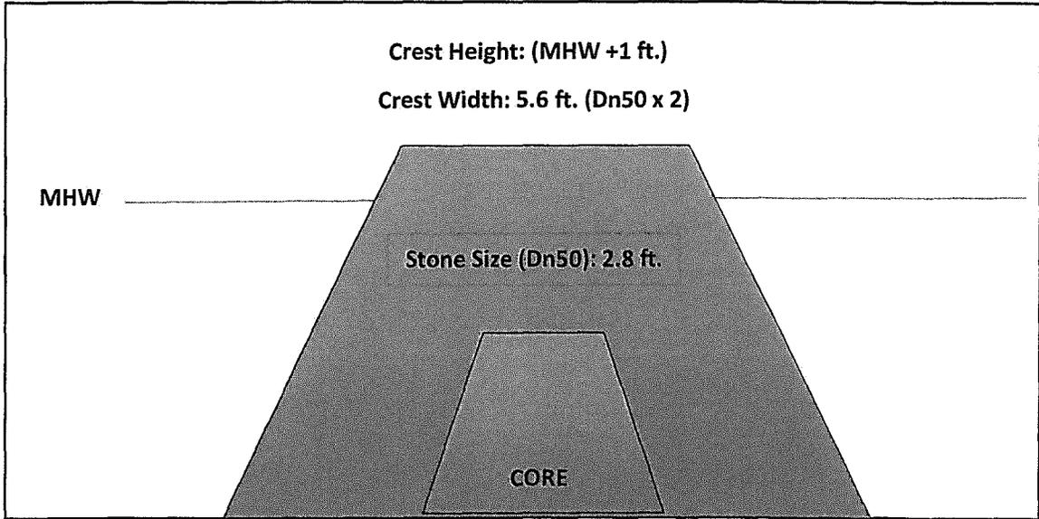
Figure 9 – Groin Cross-Section Design
