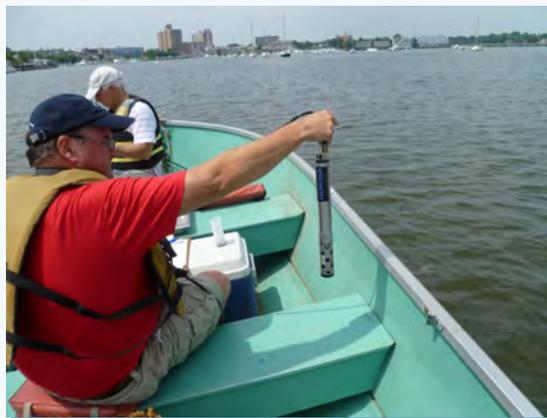
Figure O-2b. Horiba Model 4000 water quality data logger
