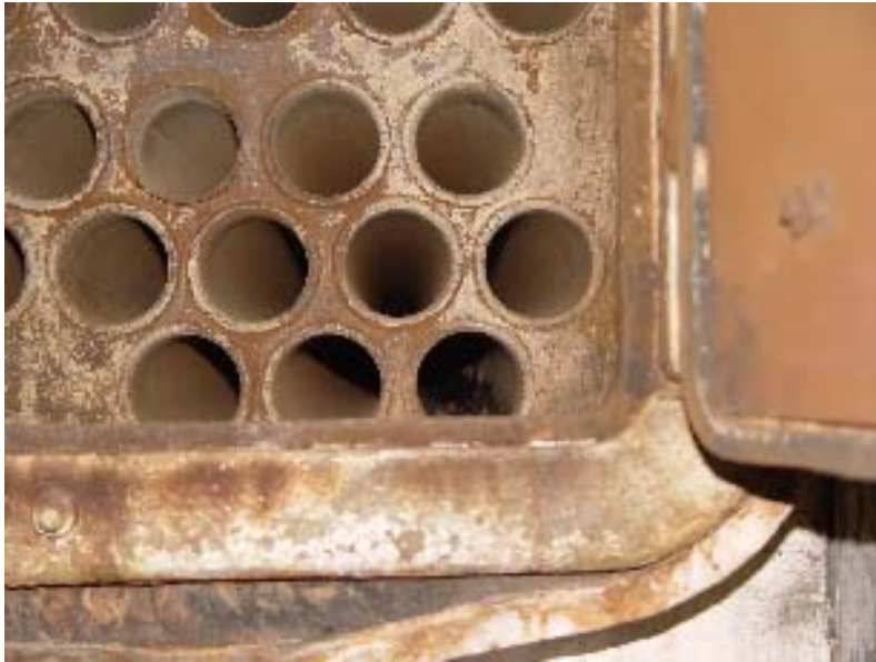
Location of Failed Tube
