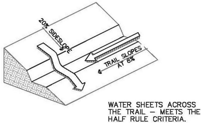
FIGURE 7. HALF SLOPE CRITERIA FOR TRAIL DESIGN
