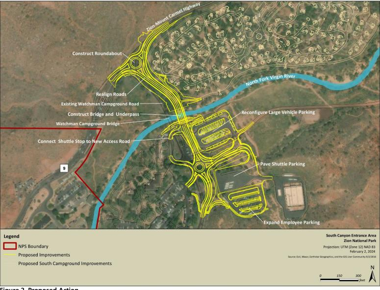
Grading would occur throughout the project area. Specifically, the new bridge would require extensive grading for installation and to connect adjacent roads and parking areas. The shuttle bus charging lot would require fill to meet grades and to tie into adjacent roads.
